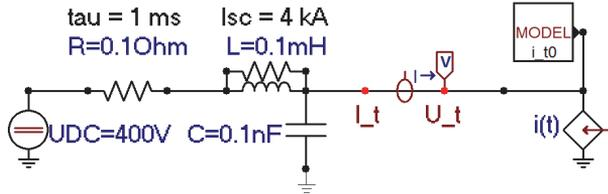
**Figure 5:** ATPDraw circuit containing a current source controlled by a predefined current time function
