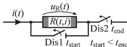
**Figure 1:** Schematic of switching device with time-dependent resistor
