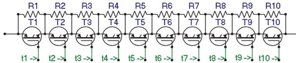
Figure 9: Many power-semiconductor switches in switch-off mode, each with a parallel connected resistor in series
