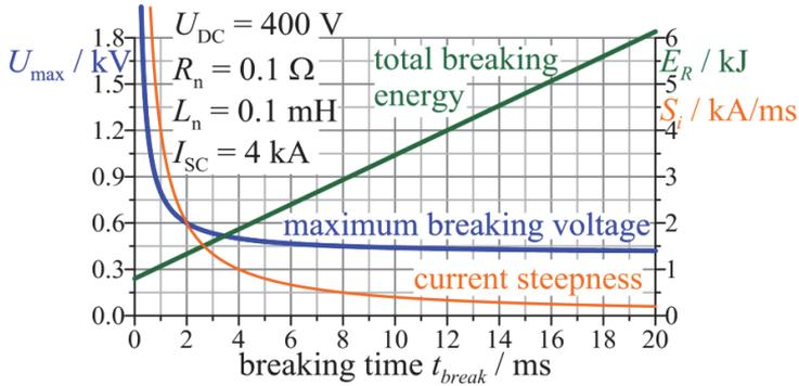
**Figure 7:** Relation between maximum breaking voltage, total breaking energy, and breaking time for a linear decaying current
