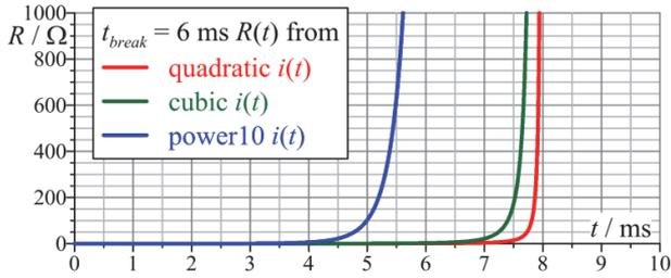
Figure 8: Variable resistance rise using ATP with respect to time
