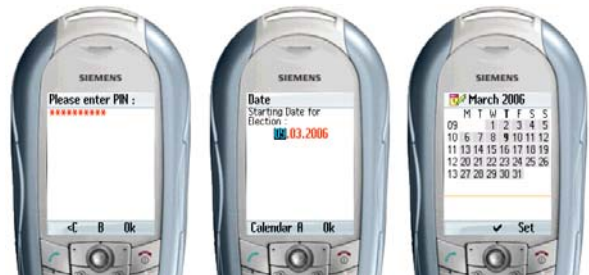
Figure 5: Wireless Java provides standard UI elements for simplified application programming. The samples here show how password input can be masked automatically, and how comfortable the input of date information can be.
