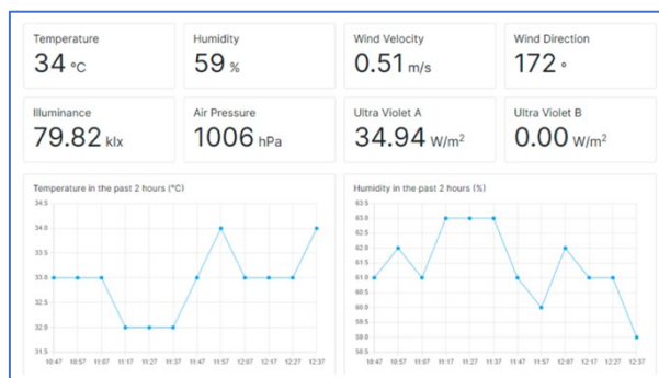
Figure 8: The dashboard interface used in the web application Source: own.
