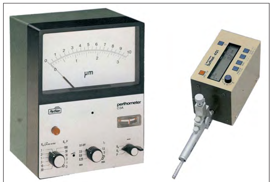
Figure 14. Measuring device SURFTEST 401 - 2MITUTOYO 2
