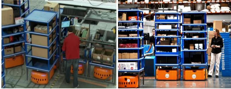
Fig. 14 Service robots – KIVA systems [23]
