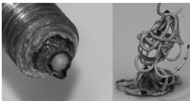
**Figure 6:** Degradation of PEEK inside the nozzle as a result of several heating cycles. The left figure shows the inside of the nozzle after being used for 15 cycles (15 working days). The right figure shows small particles that are caused by the material degradation inside the nozzle and are eventually deposited onto the product.
