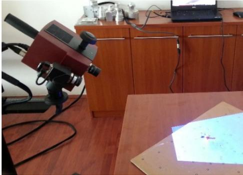
**Fig. 2** Scanning kidney stone with ATOS Compact Scan
