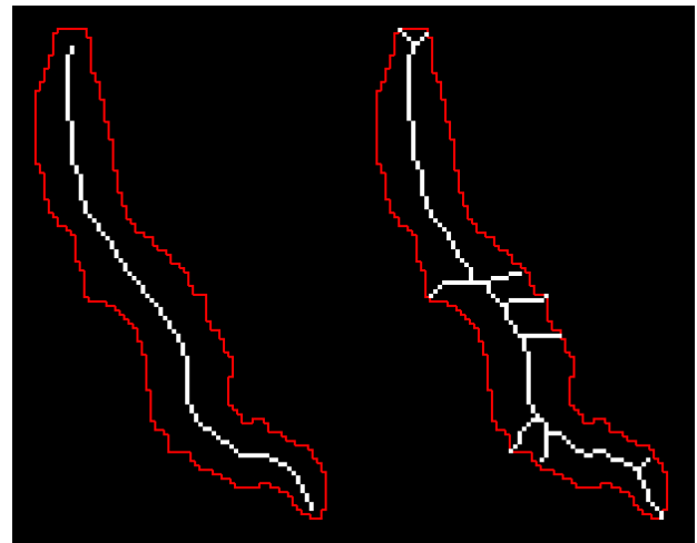
Figure 5. Illustration of the worm skeletons (white) computed from the binary segmentation image (outlined by the red line). The left skeleton was computed using the morphological thinning, the right one using skeletonization (MAT) technique.
