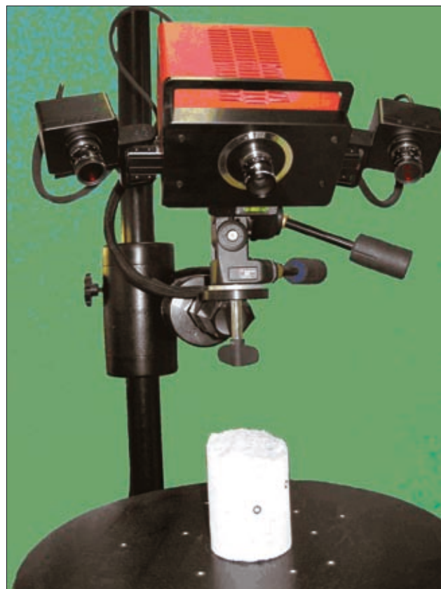
Fig. 6. The ATOS I 3D scanner and the sample Sl. 6. 3D skener ATOS I in vzorec
