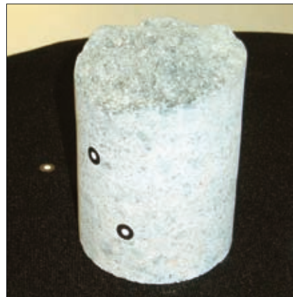
Fig. 7. A sample of tuff, with markers Sl. 7. Vzorec tufa z označbami
