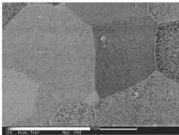
Figure 1: a) SEM image of segregated C on different grains of \alpha\text{Fe} . The sample was annealed at T < 550^{\circ}\text{C}
