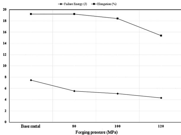
**Figure 2:** Effect of forging pressure on elongation at break and failure energy
