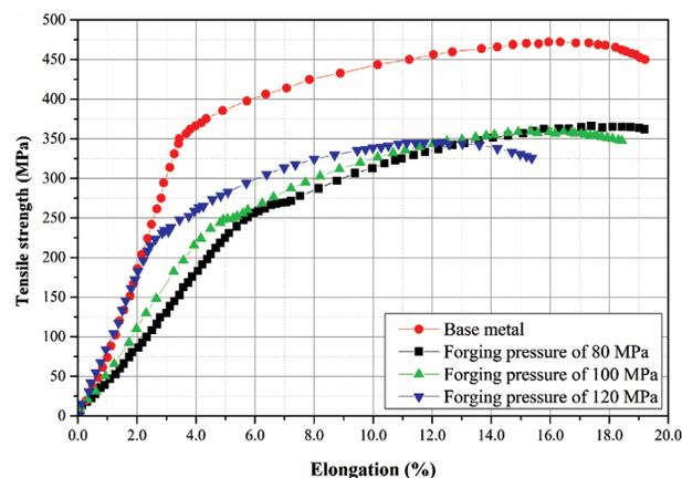
**Figure 1:** Effect of different forging pressures on tensile strengths
