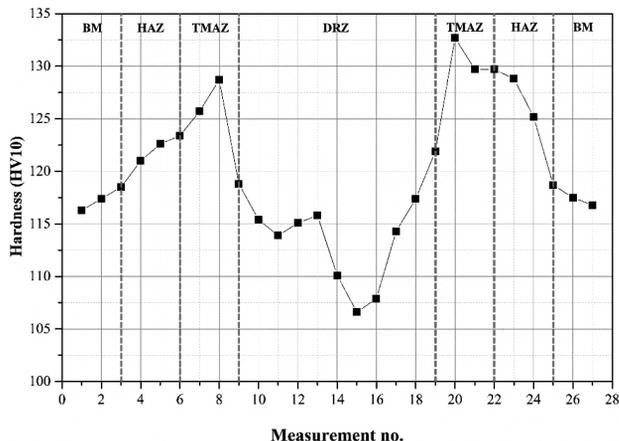
Figure 4: Line hardness measurement from cross-section of the rotary-friction-welded AA2024
