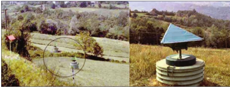
Fig. 8. Artificial rectangular permanent scatterer (TRE, 2006).
