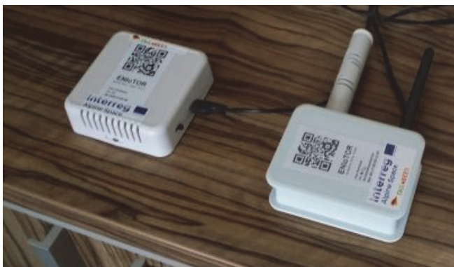
Figure 3: ENIoTOR sensor box-Arduino (left) and data concentrator-Raspberry Pi (right)
