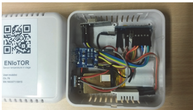
Figure 4: ENIoTOR sensor box (Source: THE4BEES project)
