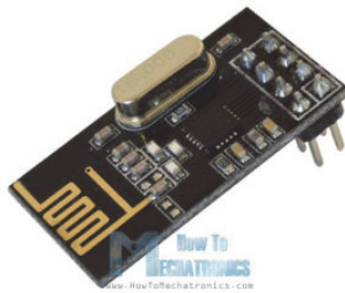
Figure 7: Wi-Fi module NRF24L01P (Source: How to mechatronics)
