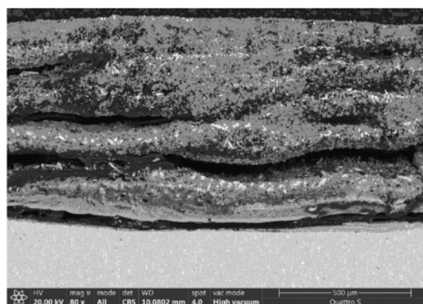
Figure 3: SEM micrograph of oxide on the surface of AISI M4 steel oxidized at 850 °C in air, a holding time of 6 h
