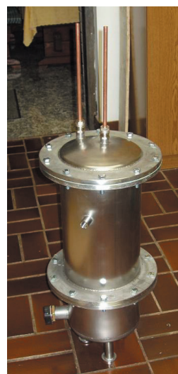
Fig. 10. Heat storage tank
