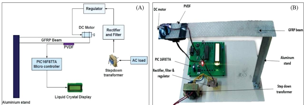
**Figure 6:** a) Schematic diagram of smart piezo-enabled GFRP beam, b) Experimental arrangement
