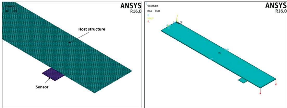
**Figure 5:** Meshed model and the applied boundary conditions
