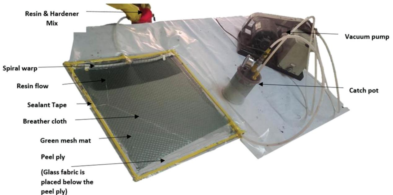
**Figure 3:** Laminates preparation using vacuum-assisted infusion technique
