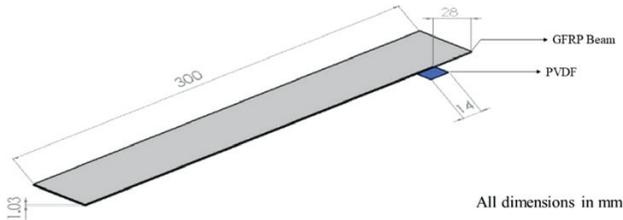
**Figure 2:** Structural geometry of piezo-enabled GFRP beam structure
