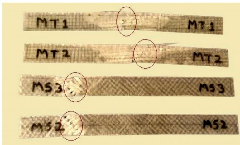
**Figure 4:** GFRP Test coupons after mechanical testing
