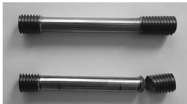
Figure 7: A test specimen of CVC NiTi rod before and after the tensile test
