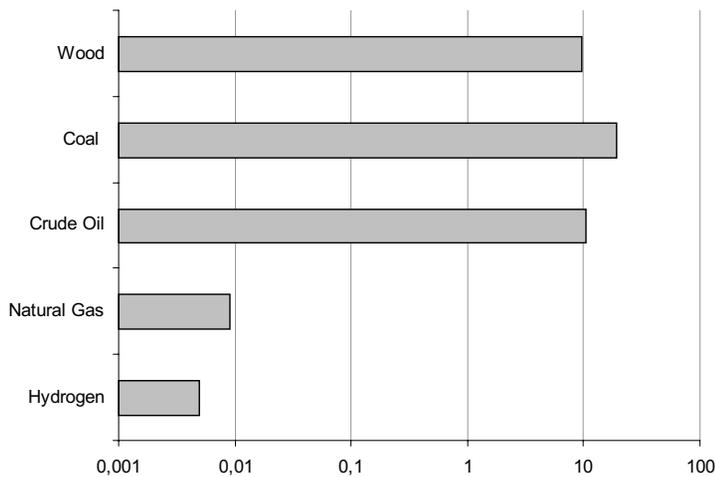
Fig. 3. *Volumetric energy density of some common fuels*
