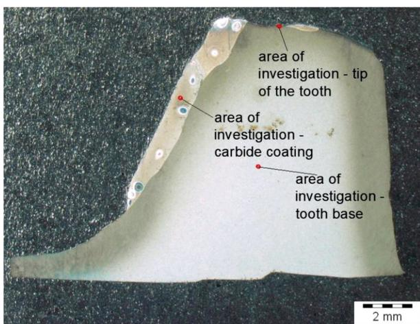
**Figure 5:** Vickers hardness testing areas
