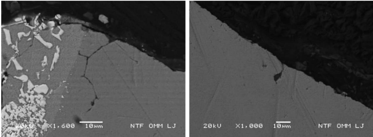
**Figure 8:** a) Microcracks at the interface between the carbide coating and the tooth steel, b) erosion channel
