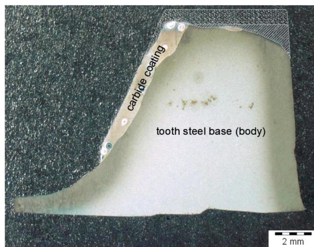
**Figure 3:** Cross-section of the tooth with reconstruction of the worn part
