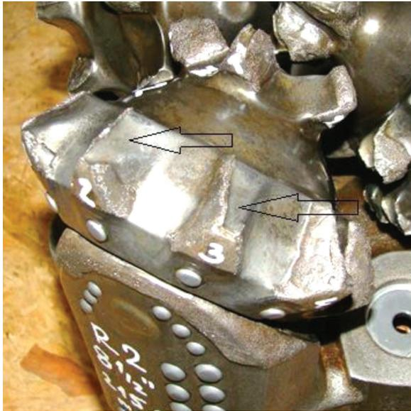
**Figure 6:** Overview of the characteristic wear of the teeth of a roller-cone drill bit 117
