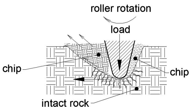
**Figure 1:** Advance of the tooth into the rock
