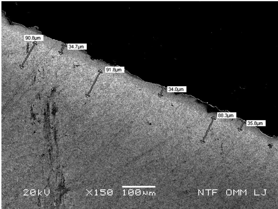
Figure 10: Temperature-influenced area of the tooth of the roller-cone drill bit 136
