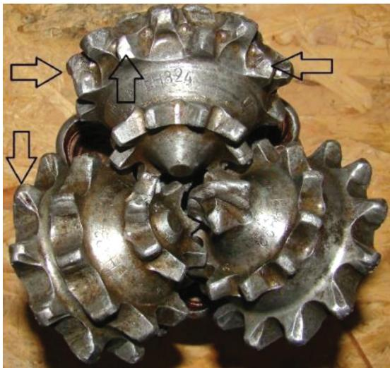
**Figure 7:** Overview of the characteristic wear of the teeth of a roller-cone drill bit 136
