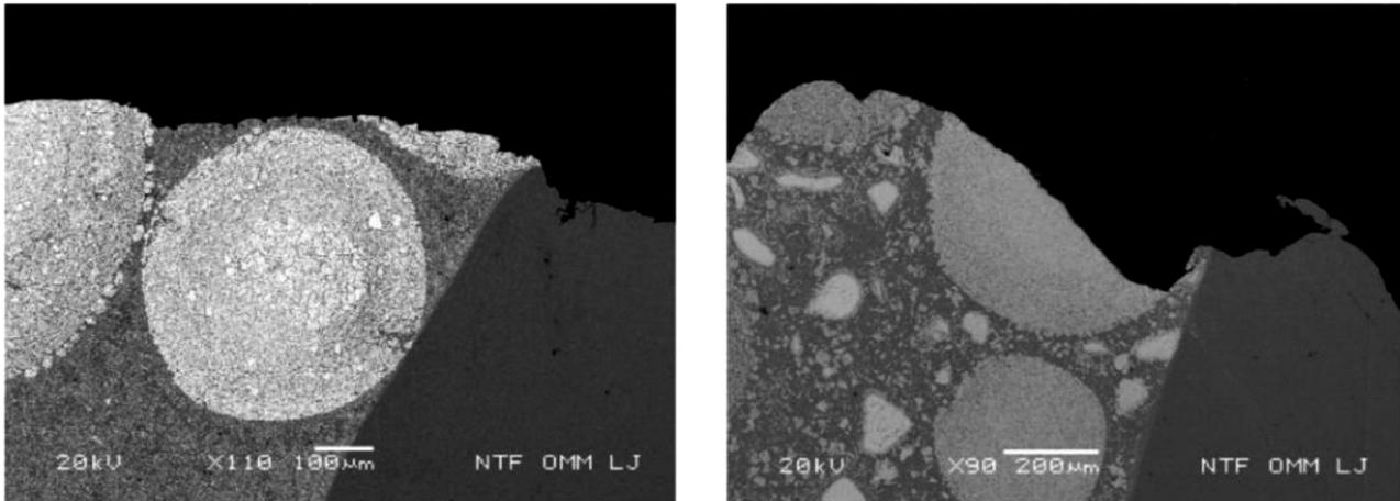
**Figure 4:** Carbide coating. The layer that protects the tooth surface from erosion (a) bit 136, b) bit 117)
