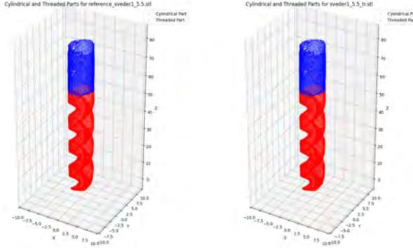
Figure 3: Extraction of the Cylindrical and Threaded Parts of Milling Cutters
