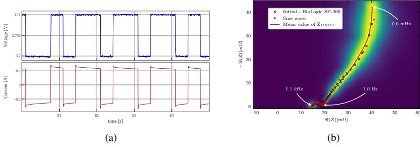
Figure 1: EIS measurement with DRBS on lithium-ion battery [1]. a) Time domain of the voltage excitation and the current response of the battery. b) Comparison of impedance calculated using DRBS and classical single-sine excitation signals..
