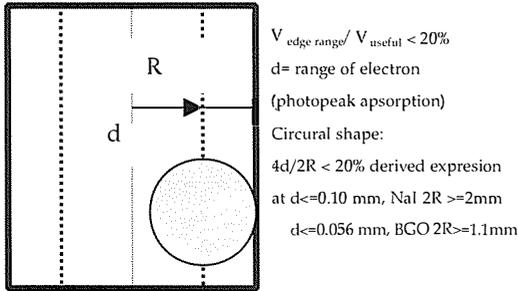
**Figure 2.** An estimate of the limit for the crystal cross sectional size. The shadow region represents the volume of induced ionization and the place from which the scintillation light contributes to the energy signal. The data for stopping power of electrons were taken from.<sup>1</sup>
