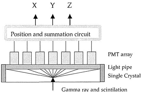
**Figure 1a.** Imaging detector with a single large scintillation crystal with set of PMTs.
