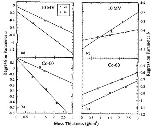
**Figure 5.** Plots of regression parameters  $a$  and  $b$  versus detector front-plate mass thickness. A linear relationship exists between the regression parameters and the mass thickness for a given metal, and parameters for the linear fits are given in Table 3.
