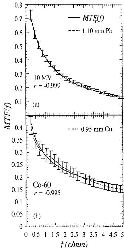
**Figure 4.** The  $MTF(f)$  data and the calculated ( $MTF_L(f)$ ) are shown for (a) typical case with  $r = -0.999$  and for the (b) worst case with  $r = -0.995$ .
