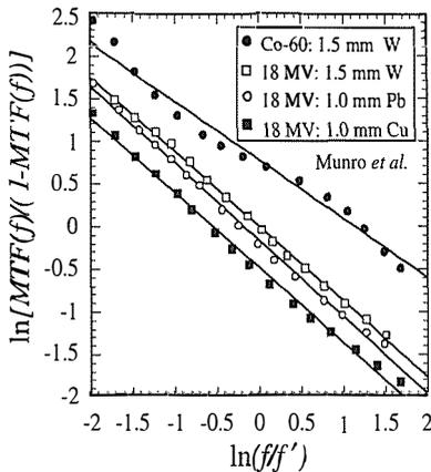
**Figure 3.** Logit fits to the  $MTF(f)$  data from the literature [Munro et al. ref(7)]. The straight lines are the logit  $MTF$ 's calculated using the regression parameters in Table 2. For clarity, the curves for 1.5 mm W at Co-60 and 1.0 mm Cu at 18 MV were displaced vertically by 0.5 and -0.25, respectively.
