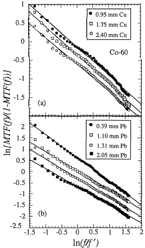
**Figure 1.** Logit fits to the *MTF(f)* data collected with the 10 MV spectrum for the detectors with (a) Cu, and (b) Pb front-plates. The straight lines are the logit *MTF*'s calculated using the regression parameters in Table 1. For clarity, the curves corresponding to the 2.40 mm Cu, 0.39, and 1.10, 2.05 mm Pb front-plates were displaced vertically by -0.5, 0.5, 0.5, and -0.5, respectively.
