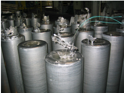
Fig. 6. Billet instrumented with thermocouples for temperature measurement
