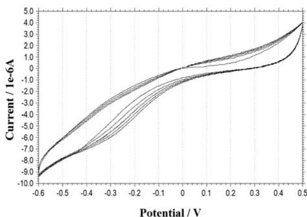
**Figure 1.** Cyclic voltammogram of Fe-EHPG complexes (**2b–2e**) in 100 mmol/L phosphate buffer pH = 7.4.
