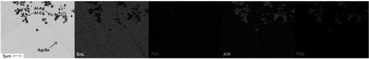
**Figure 5:** Scanning elemental maps of the Sn-1Ag-0.5Cu-0.2Al
