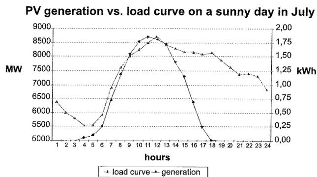
Fig. 2: PV generation versus typical load /2/
