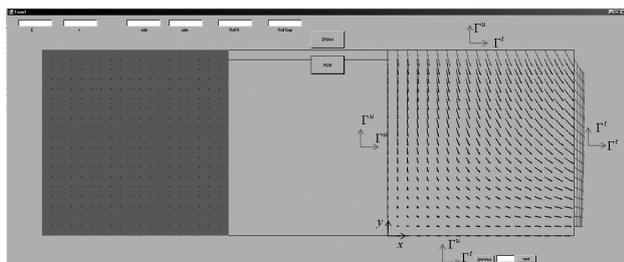
**Figure 3:** Simulation of flat rolled (180 × 180) mm cross sectioned 16MnCrS5 steel at 1100 °C with Young's modulus  $E = 97362.21$  MPa and Poisson's ratio  $\nu = 0.35678$ . The total reduction is 16.66 % and preliminary analyzed with 5 slices by using elastic stiffness matrix <sup>7</sup>. Arrows represents the displacement vector for each slice. The exit speed is equal to 1.14389 times the entry speed of the billet. Due to symmetry only the top right part of the billet is considered.
