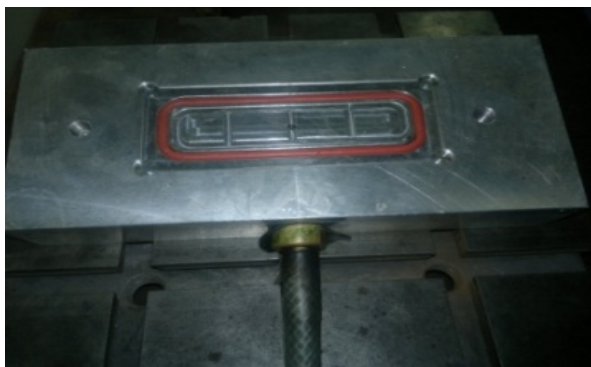
Fig. 2 Shop made vacuum fixture used for experiments [19]
