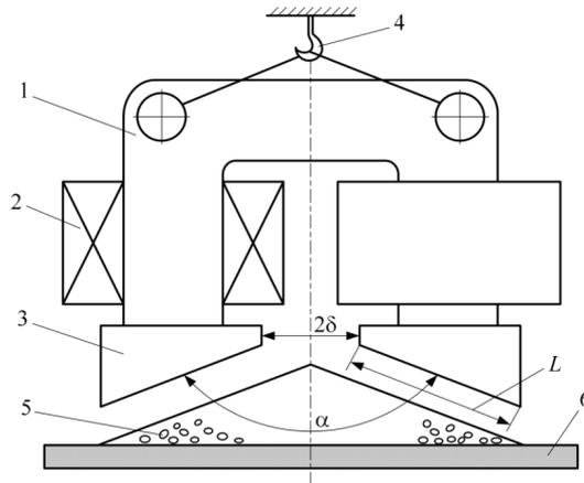
**Figure 1:** Suspended electromagnetic separator
