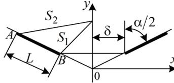
**Figure 3:** Two plane-parallel plates having the angle  $\alpha$  between their surfaces
