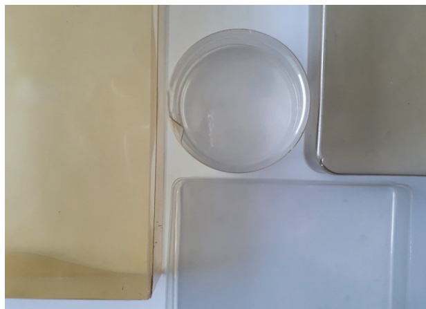
Figure 7: Discolouration of PVC objects.
