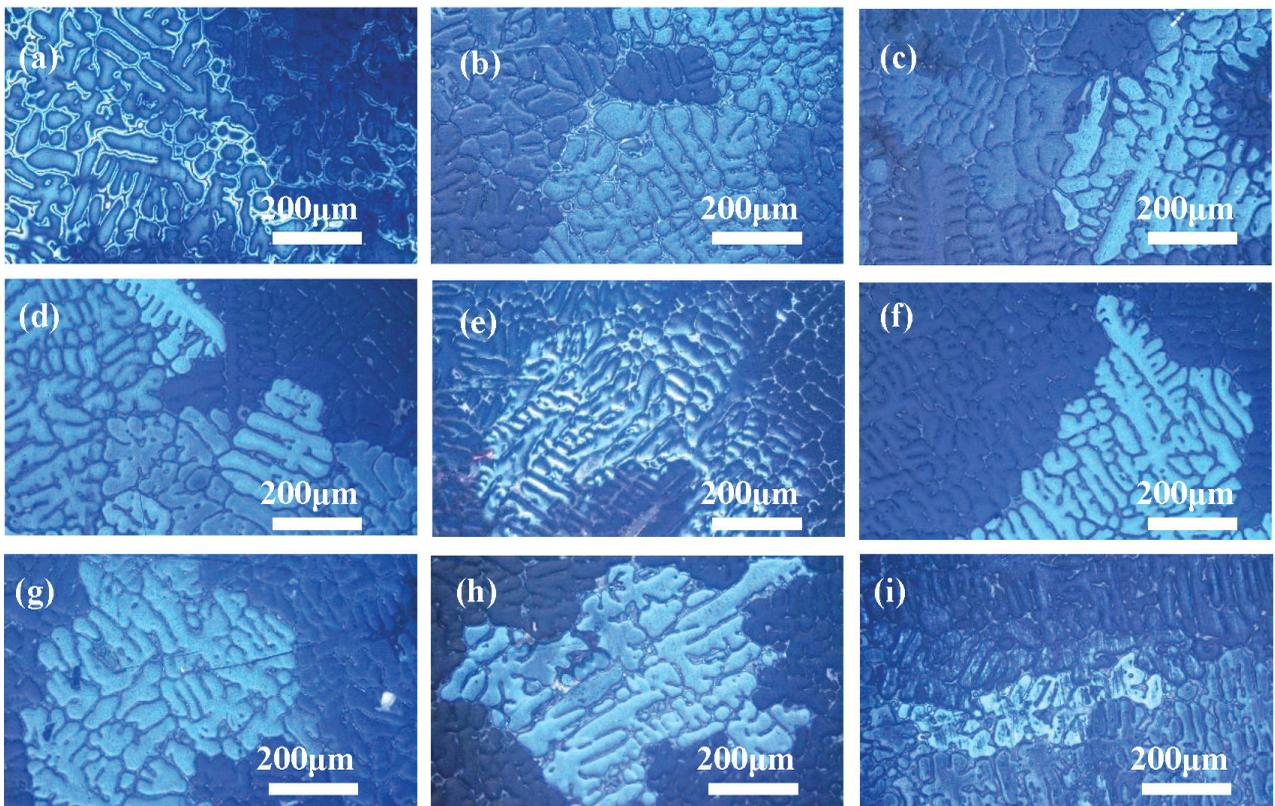
**Figure 6:** Microstructure of the Al-5Cu alloy ingot without forced water cooling but with ultrasonic treat. for 90 s: position 1, b) position 2, c) position 3, d) position 4, e) position 5, f) position 6, g) position 7, h) position 8, i) position 9
