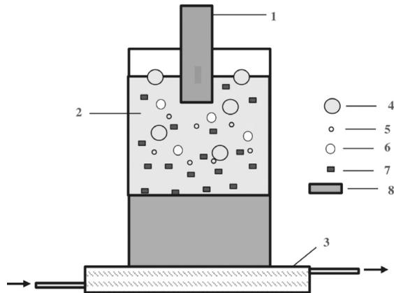
**Figure 12:** Schematic diagram of aluminum alloy with ultrasonic degassing: 1 – ultrasonic probe, 2 – aluminum, 3 – copper plate in water, 4 – cavitation bubbles formed by ultrasonic treatment, 5 – gas in the melt, 6 – hydrogen diffuses into cavitation bubbles, 7 – refined equiaxed grains, 8 – forced cooling zone
