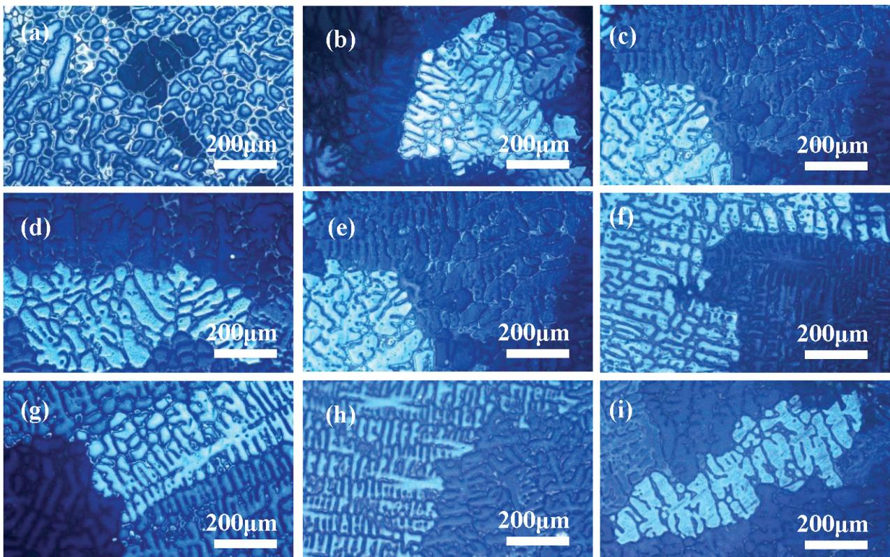
**Figure 4:** Microstructure of the Al-5Cu alloy ingot after normal cooling: a) position 1, b) position 2, c) position 3, d) position 4, e) position 5, f) position 6, g) position 7, h) position 8, i) position 9
