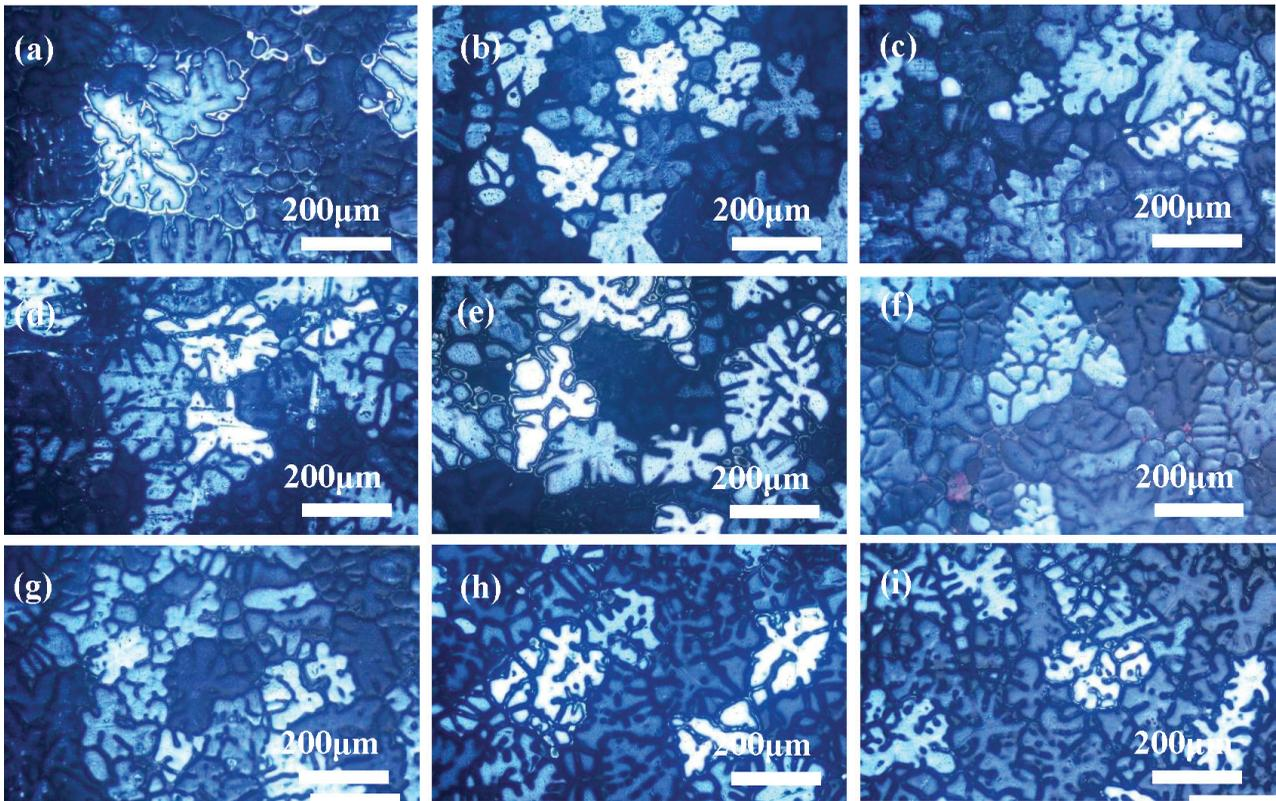
**Figure 9:** Microstructure of the Al-5Cu alloy ingot under forced water cooling and ultrasonic treatment for 150 s: position 1, b) position 2, c) position 3, d) position 4, e) position 5, f) position 6, g) position 7, h) position 8, i) position 9
