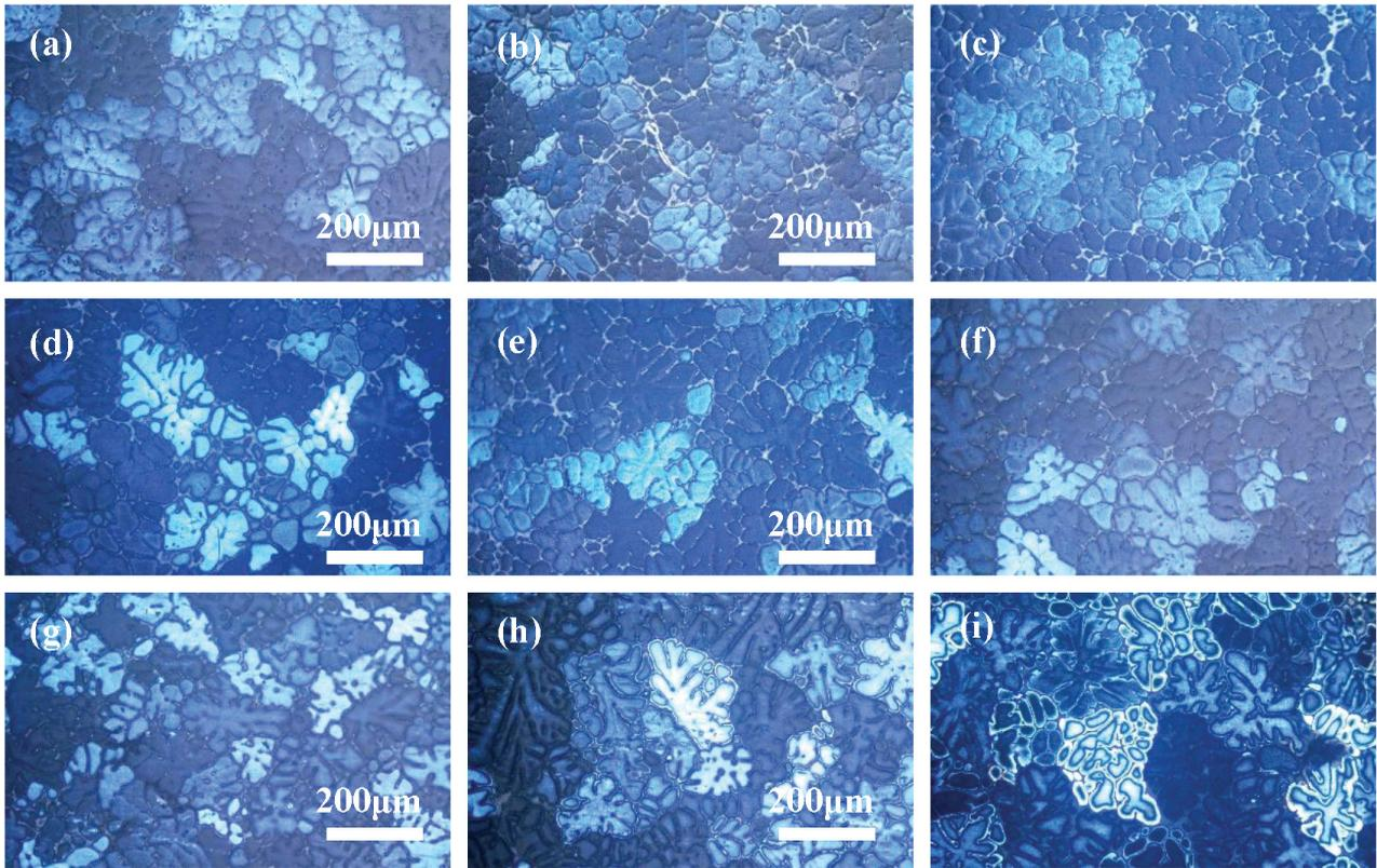
**Figure 7:** Microstructure of the Al-5Cu alloy ingot after forced water cooling and ultrasonic treat. for 90 s: position 1, b) position 2, c) position 3, d) position 4, e) position 5, f) position 6, g) position 7, h) position 8, i) position 9
