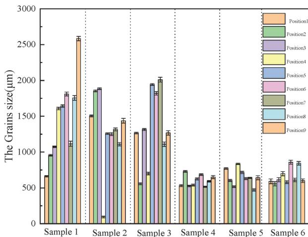
**Figure 10:** Grain-size distribution of Al-5Cu alloy ingots after ultrasonic treatment
