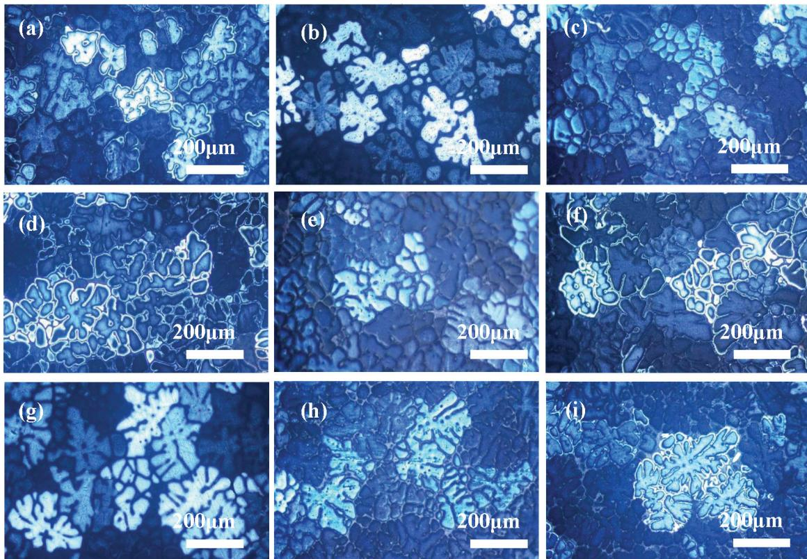
**Figure 8:** Microstructure of the Al-5Cu alloy ingot after forced water cooling and ultrasonic treat. for 120 s: position 1, b) position 2, c) position 3, d) position 4, e) position 5, f) position 6, g) position 7, h) position 8, i) position 9
