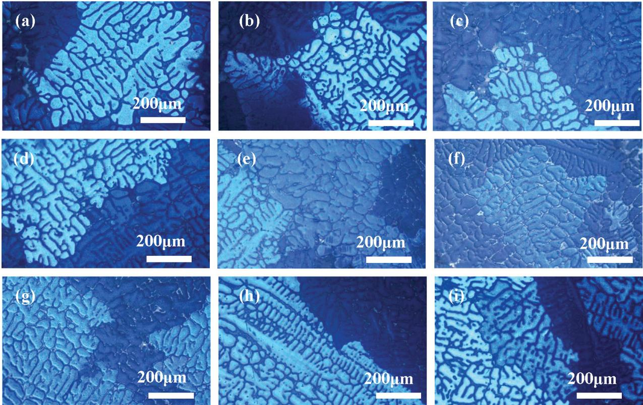
**Figure 5:** Microstructure of the Al-5Cu alloy ingot after forced water cooling: position 1, b) position 2, c) position 3, d) position 4, e) position 5, f) position 6, g) position 7, h) position 8, i) position 9
