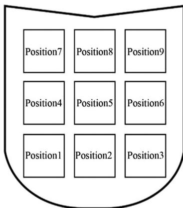
**Figure 2:** Sampling positions of Al-5Cu alloy ingots
