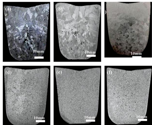
**Figure 3:** Macrostructures of Al-5Cu alloy ingots with or without ultrasonic treatment: a) normal cooling, b) forced water cooling, c) without forced water cooling but with ultrasonic treat. for 90 s, d) forced water cooling and ultrasonic treat. for 90 s, e) Forced water cooling and ultrasonic treat. for 120 s, f) Forced water cooling and ultrasonic treat for 150 s
