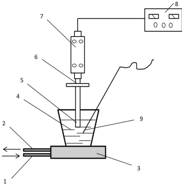
**Figure 1:** Schematic layout of the ultrasonic field device: 1 – water inlet; 2 – water outlet; 3 – copper plate; 4 – Al-5Cu alloy melt; 5 and 6 – ultrasonic probe; 7 – ultrasonic transducer; 8 – ultrasonic generator; 9 – thermocouple
