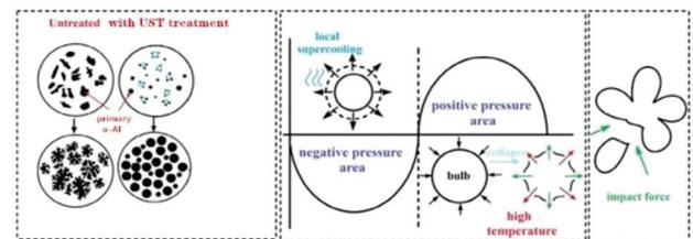
**Figure 11:** Schematic of grain refinement
