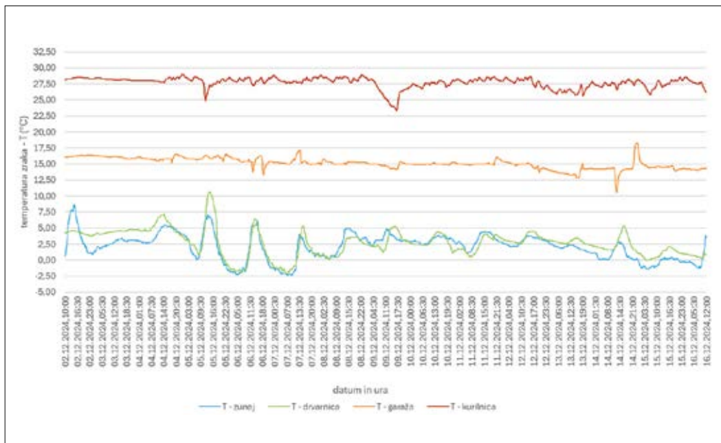
Slika 1: Temperatura na vseh lokacijah shranjevanja vzorcev lesnega oglja in briketov lesnega oglja Figure 1: Temperature at all storage locations for charcoal and charcoal briquette samples
