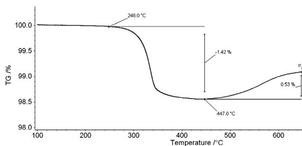
**Figure 6:** Heating TG curve of alloy A, protective atmosphere of N<sub>2</sub> 5.9, flow of 10 mL/h, 1 × vacuum,  $T_{\max} = 650$  °C, 5 °C/min
