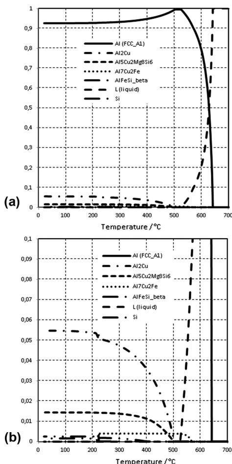
**Figure 3:** a) Theoretical equilibrium thermodynamic phase stability of alloy A and b) detail of the diagram up to a fraction of 0.1 mol, calculated with ThermoCalc<sup>3</sup>
