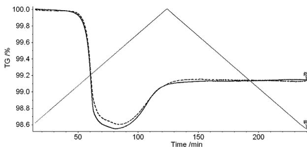
**Figure 5:** Measuring protocol of the TG analysis of alloy A (heating/cooling is presented as a fine dotted line), comparison of the TG curves obtained during the experiment performed in stationary Ar (dashed line) and the flow of N<sub>2</sub> (full line)
