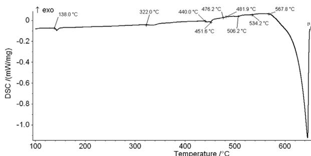
**Figure 2:** Heating part of the DSC curve of alloy A, protective atmosphere of N<sub>2</sub> 5.9, flow of 10 mL/h, 1 × vacuum,  $T_{\text{max}} = 650$  °C, 5 °C/min
