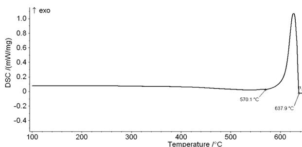
**Figure 4:** Cooling DSC curve of alloy A, protective atmosphere of N<sub>2</sub> 5,9, flow of 10 mL/h, 1 × vacuum, T<sub>max</sub> = 650 °C, 5 °C/min
