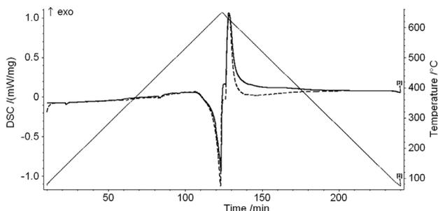
**Figure 1:** Measuring protocol of the DSC analysis of alloy A (heating/cooling is shown with a fine dotted line), a comparison of the DSC curves obtained during the experiments performed in stationary Ar (dashed line) and in a flow of N<sub>2</sub> (full line)
