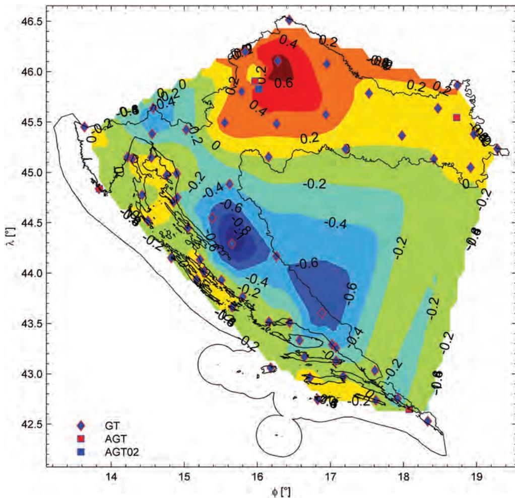
Figure 6: Spatial distribution of differences of gravity values between B and A in  $\mu\text{m/s}^2$ . The extreme negative differences are in the Dinaric Alps region with higher altitudes, for which the closest fixed gravity values are close to the sea level, while the extreme positive differences are in the northern part, where the closest fixed gravity value is at AGT03 on the mountain Medvednica.
