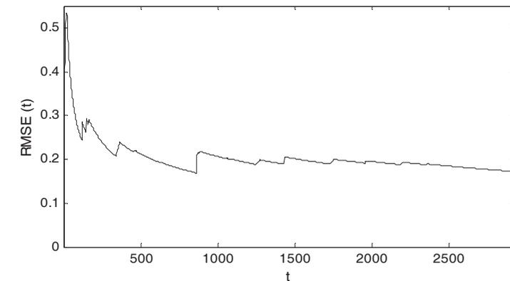
Figure 5. Root Mean Square Error (RMSE) of EFuNN model prediction on the training set
