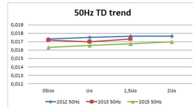
**Figure 12:** Trending results for  $\tan \delta$  at power frequency 50Hz
