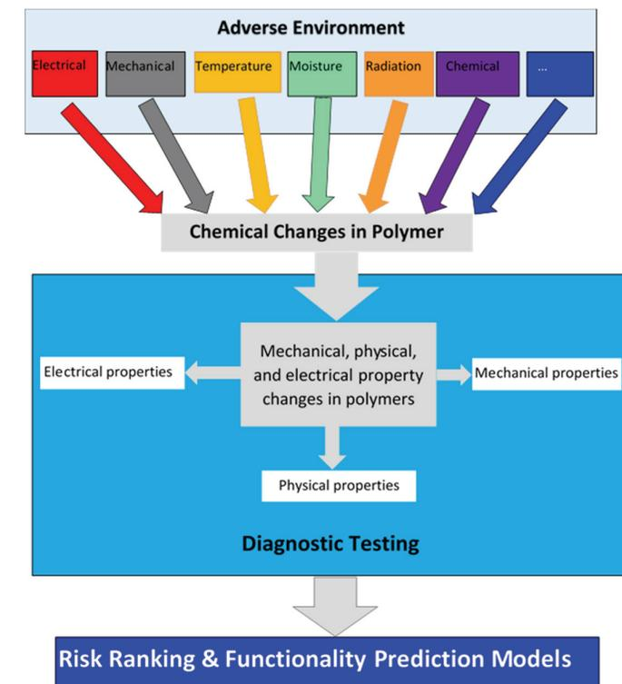
Figure 2: Cable Aging Detection and Remaining Life Prediction, [4]
