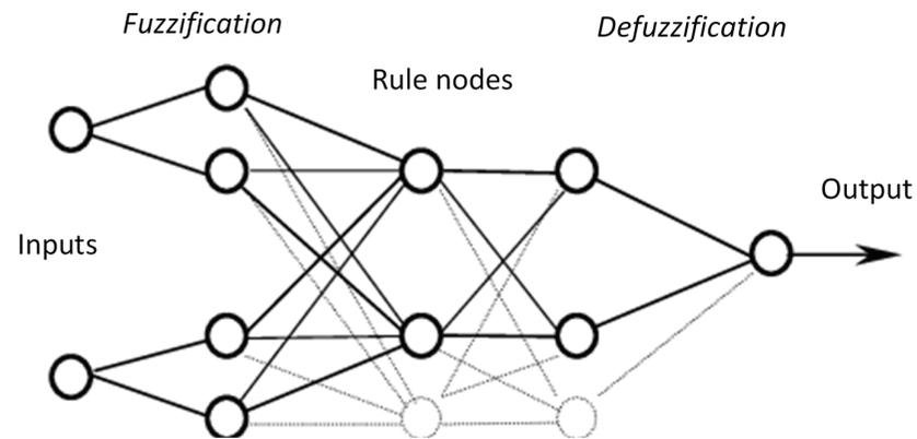
Figure 4. Architecture of Evolving Fuzzy Neural Network (EFuNN)
