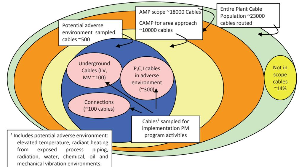
Figure 1: Cable scoping and sampling process, [1]
