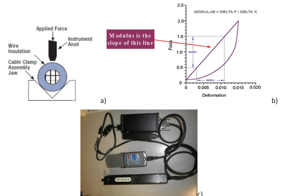
**Figure 4:** Indenter Modulus Testing Equipment and functionality description, [6]
