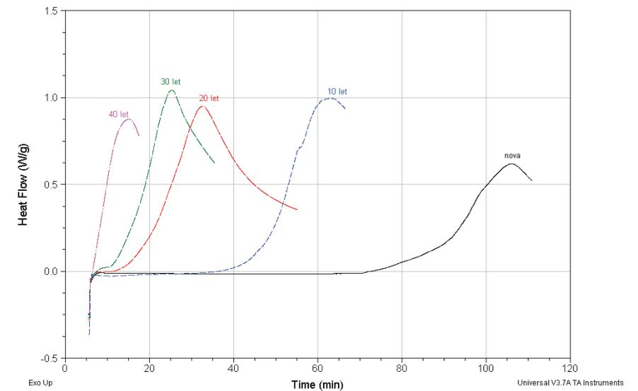
Figure 10: DSC Heat Flow of different aged cables [9]
