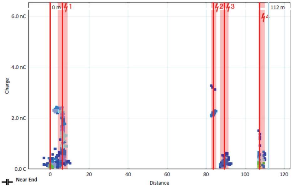
Figure 15: Significant PD events: XLPE cable failure at 5 m from cable near end
