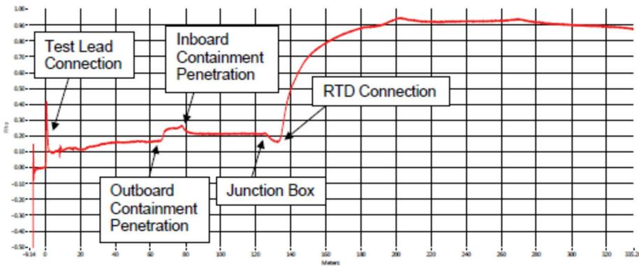
Figure 14: TDR test plot with route configuration description, [9]
