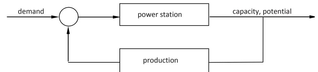
Figure 1: Regulation circuit of the power supply system
