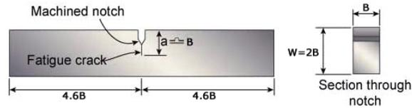
Figure 2: Fracture mechanics SENB specimens with  $B=15$  mm
