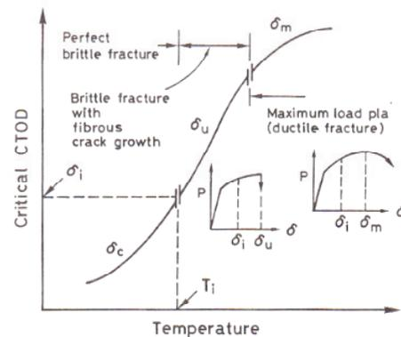
Figure 4: Definition of critical CTODs in ASTM E1290-08e1.
