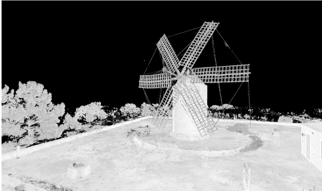
operations using Agisoft Metashape software from sets of images taken by drone; these point clouds, once aligned with the ones obtained by laser scanning, made it possible to produce an almost complete digital copy of the analysed structures.
