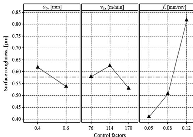
Figure 7: Mean effect plots for  $R_a$  surface roughness
