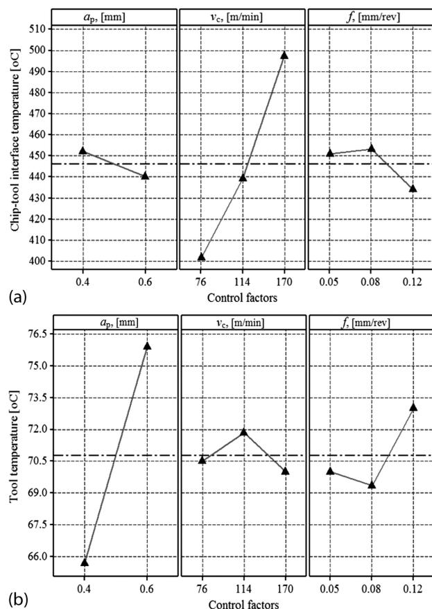
Figure 6: Mean effect plots for temperatures: a) tool-chip interface temperature, b) tool temperature
