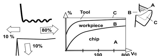
**Figure 1:** The balance of heat generation and heat dissipation during metal cutting
