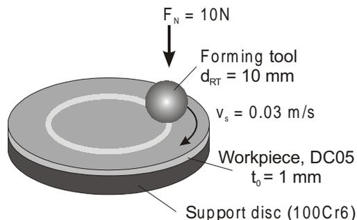
Fig. 3. Pin-on-disc test
