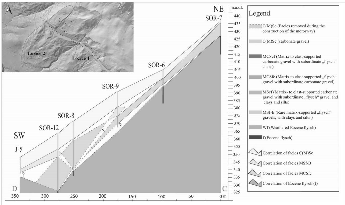
Fig. 5. Longitudinal cross-section through the Lozice 2 fossil landslide with logged facies and correlations with facies C(M)Sc, MSf-B, MCSf, and Eocene flysch. *The reader should refer to the online version of the article for the colour figure.*
