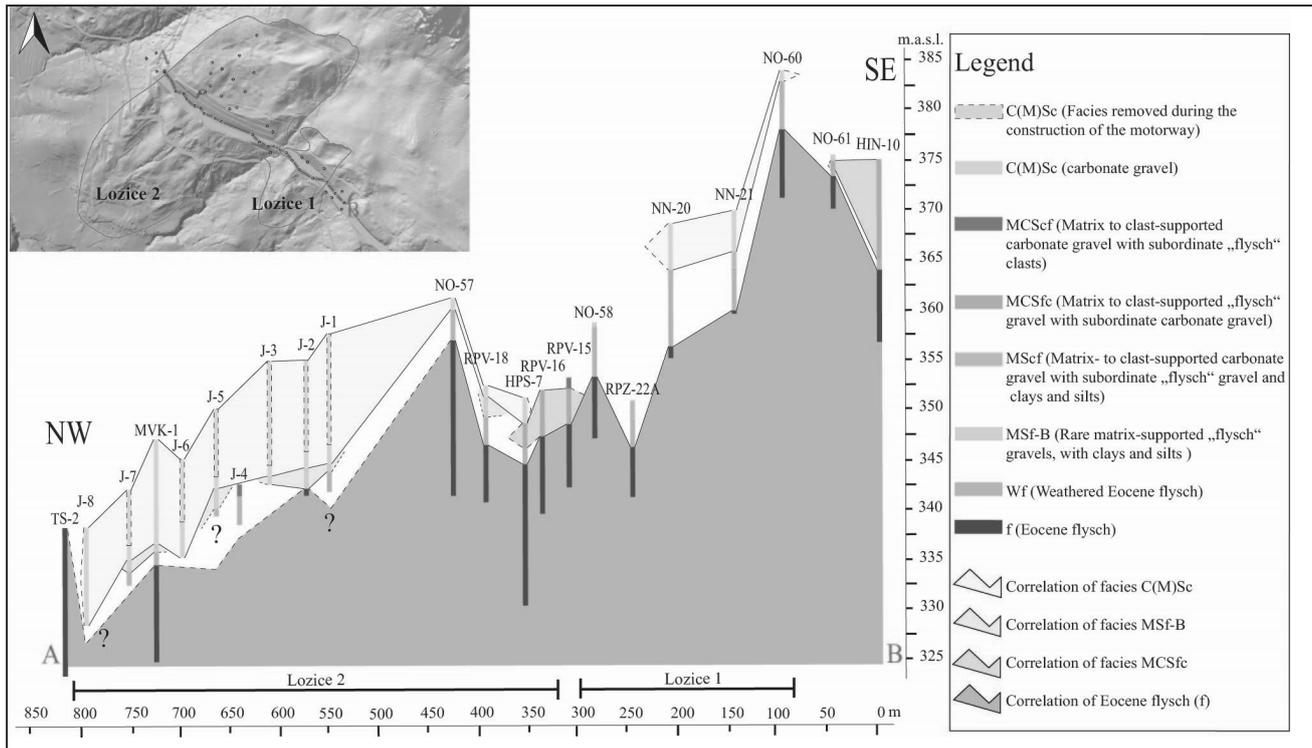
Fig. 4. Transverse cross-section through the Lozice fossil landslide with logged facies and correlations with facies C(M)Sc, MSf-B, MCSf, and Eocene flysch. *The reader should refer to the online version of the article for the colour figure.*
