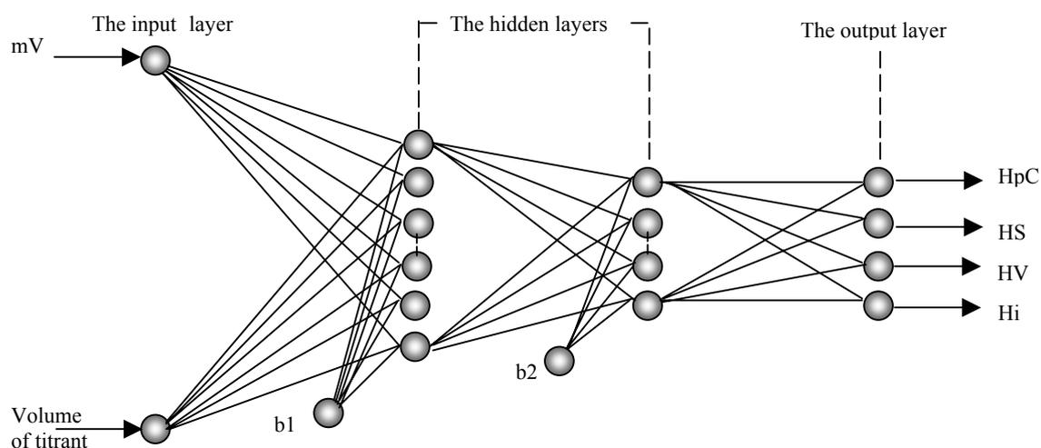
Figure 1. Network architecture used in the potentiometric titration modeling.
