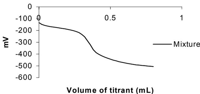
**Figure 3.** Titration curves equimolar quaternary mixtures with tetrabutylammonium hydroxide.
