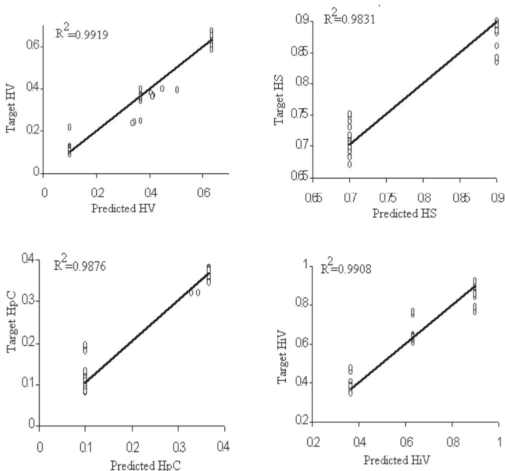
**Figure 5.** Comparison of predicted results from the NN3 model with target values from the actual values HpC, HS, HV and HiV for the testing data set.
