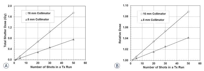
FIGURE 3. Shutter dose for the 8 and 16 mm collimators. A: The target position is the same for all measurements. Measured dose associated with PPS positioning increases with increase in the number of shots in a run and collimator size. B: The relative dose was calculated by normalizing the dose from the multiple shot plans to the single shot plan.
