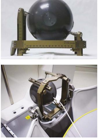
FIGURE 1. Setup of phantom for measurements. A: Framed phantom B: Phantom fixed to the PPS with a frame adaptor.
