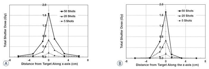
FIGURE 4. Total shutter dose for the 16 mm collimator. A: The shutter dose along the x-axis is greatest at the target site and falls off with distance; it will also increase with the number of shots. B: The shutter dose along the z-axis does not have the same symmetry as it does along the x-axis. The collimators are angled towards the inferior direction; this will increase exposure inferior to the target, as seen.
