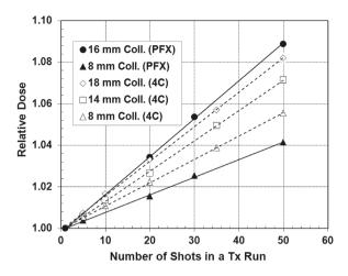
FIGURE 7. Shutter and inter-shot transit dose at the target site for the Gamma Knife® Perfexion<sup>™</sup> (PFX) and model 4C (4C), respectively. The shutter and inter-shot transit doses are not accounted for by the treatment planning system.
