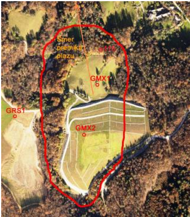
Figure 27: The scope of the landslide on the area of the Boršt site, the direction of movement of the landslide (informative), the locations of monitoring points through GPS system (points GRS1, GMX1 and GMX2) and of geodetic grid (point 115)
