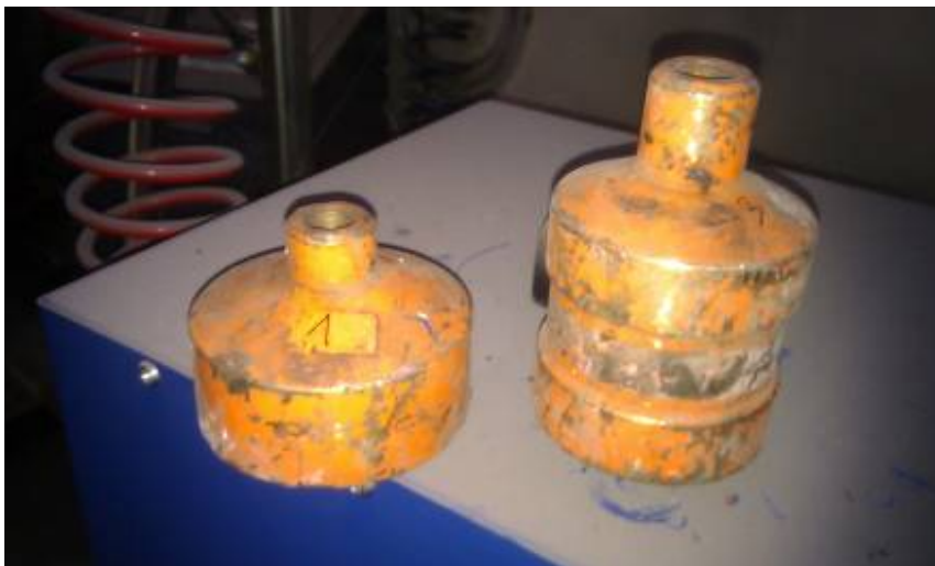
Figure 15: Collimators produced from depleted uranium
