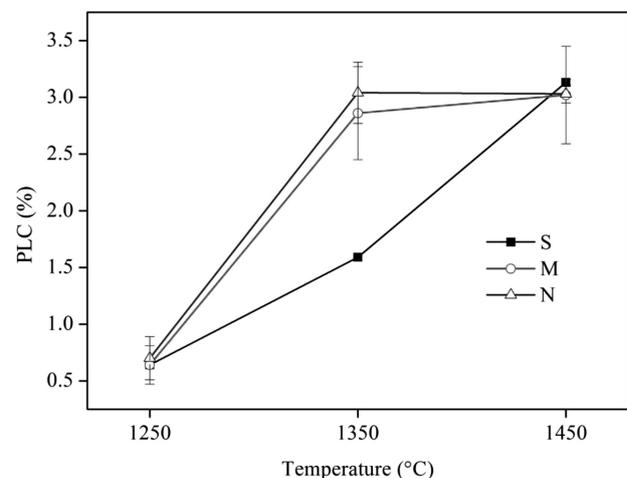
**Figure 4:** Permanent linear change of samples calcined at different temperatures
