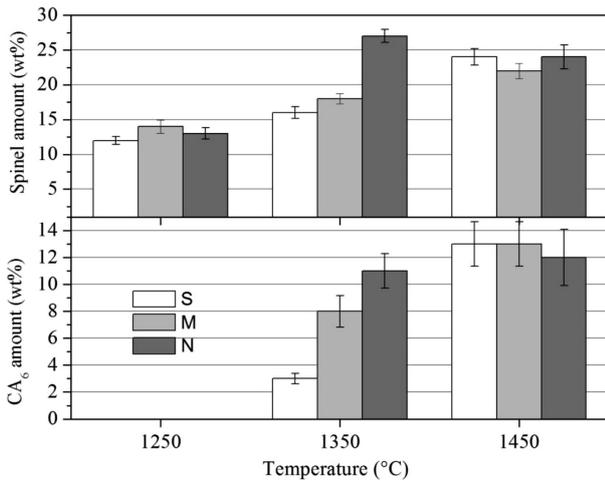
**Figure 2:** Spinel and CA<sub>6</sub> amounts for specimens calcined at different temperatures
