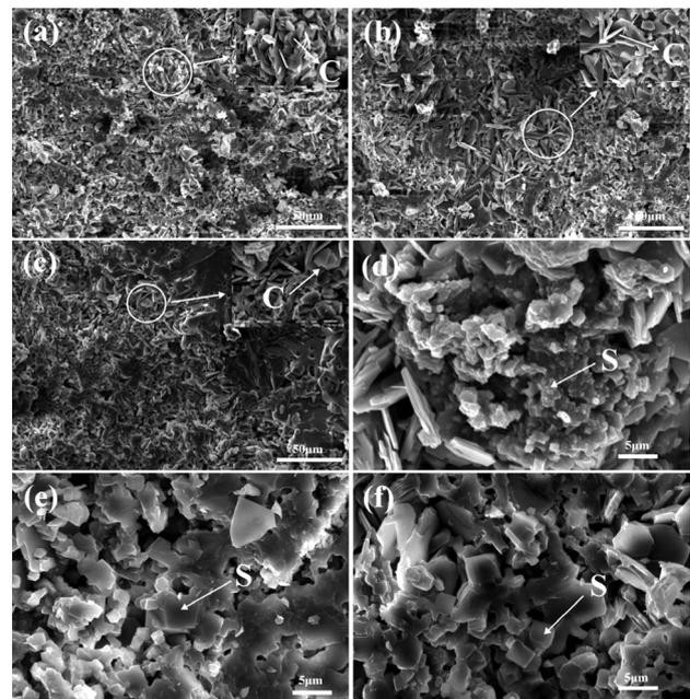
**Figure 7:** SEM images of alumina-magnesia refractory castables after treating at 1450 °C for 5 h: a)-d) S, b)-e) M, and c)-f) N (C indicates  $CA_6$  and S indicates Spinel)
