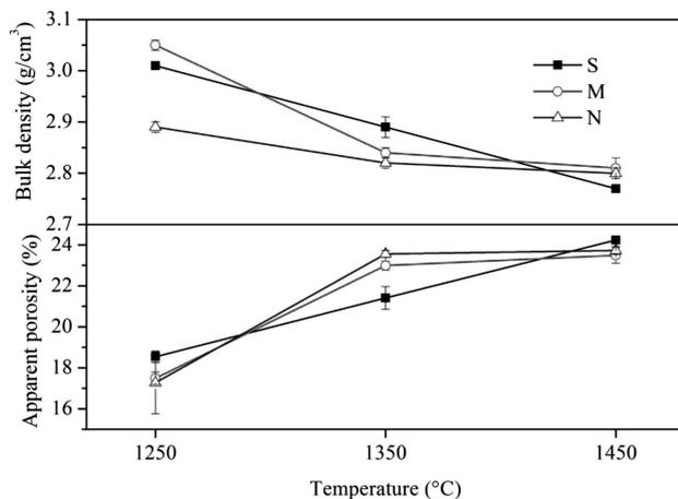
**Figure 5:** Bulk density and apparent porosity of castables treated at different temperatures
