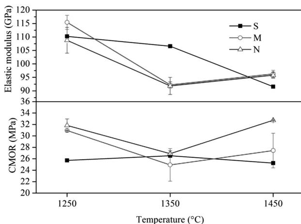
**Figure 6:** The elastic modulus and CMOR of alumina-magnesia refractory castables
