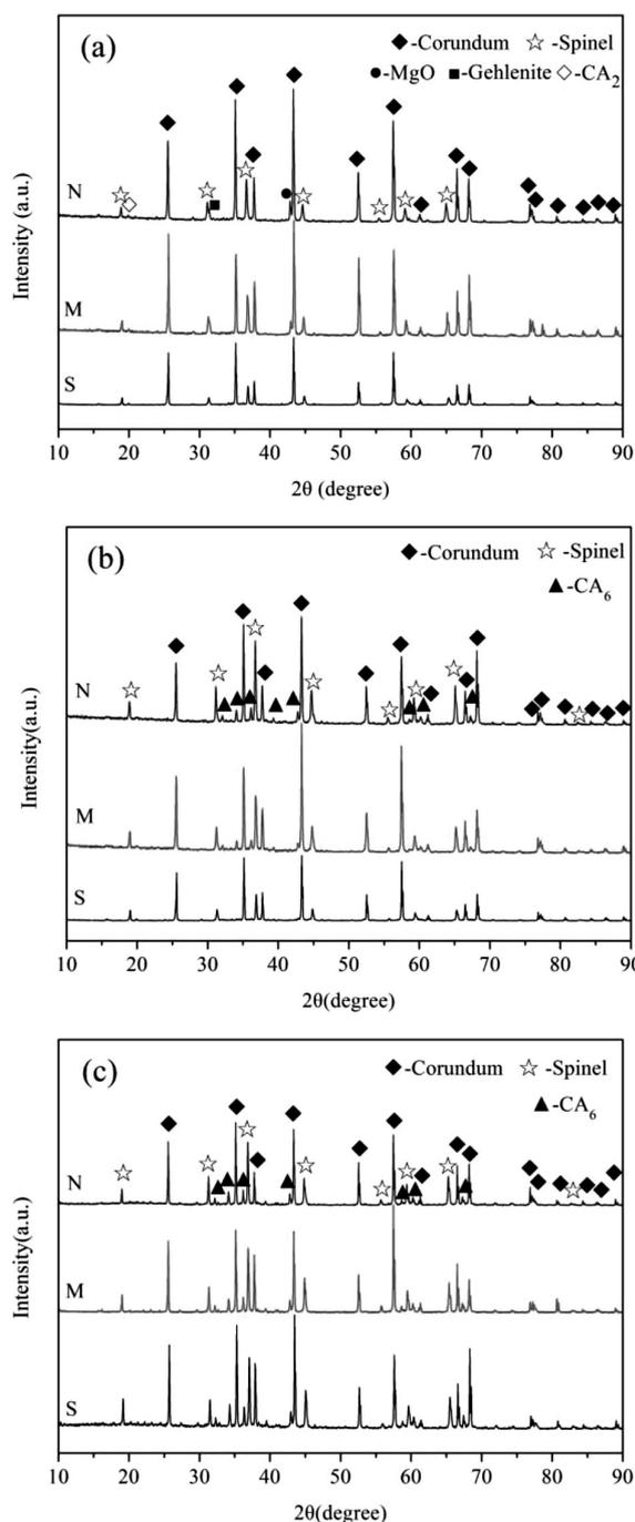
**Figure 1:** XRD patterns of alumina-magnesia refractory castables calcined at different temperatures: a) 1250 °C, b) 1350 °C and c) 1450 °C
