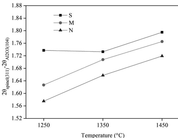
**Figure 3:** The diffraction peak shift for the spinel with the firing temperature
