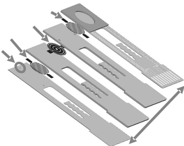
**Figure 26:** One way DSC Chip
