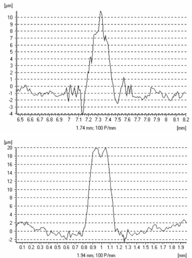
**Figure 21:** Posting effect: 10µm, new transition via compared to 20µm Conventional AgPd transition via
