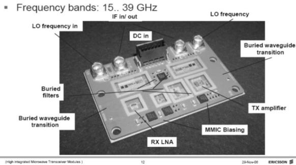
**Figure 11:** Ericsson: Modular kit of LTCC T/R modules, 15 to 39 GHz
