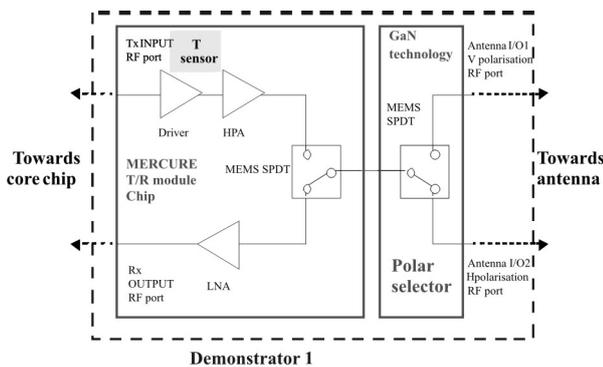
**Figure 16:** Thales: Block Diagram Wide Band T/R module
