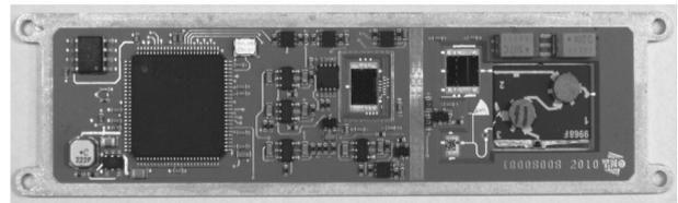
**Figure 23:** TNO: TR-Module using CarfAl heat sink
