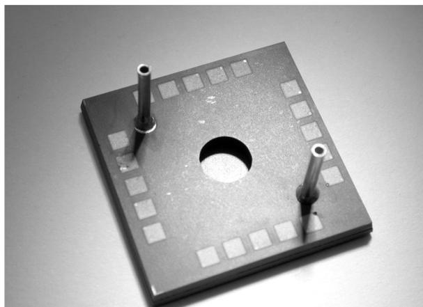
**Figure 28:** LTCC Micro reactor
