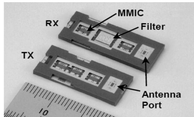
**Figure 10:** NEC 60 TX and RX Module
