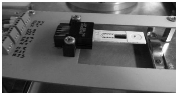
**Figure 27:** DSC Chip in test fixture (University of Bayreuth)
