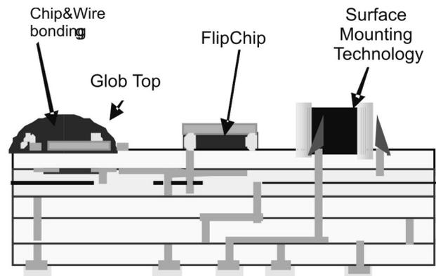
Figure 5: Epcos: Schematic of a LTCC frontend,
