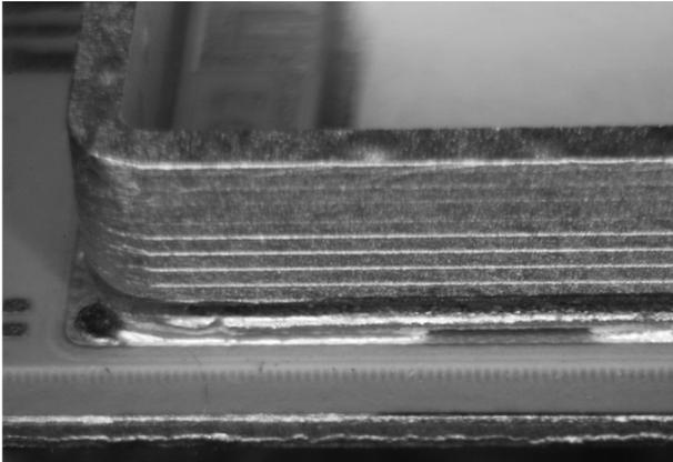
**Figure 20:** Preform Pb92.5Sn5Ag2.5 on AgPt, Carfal ring frame
