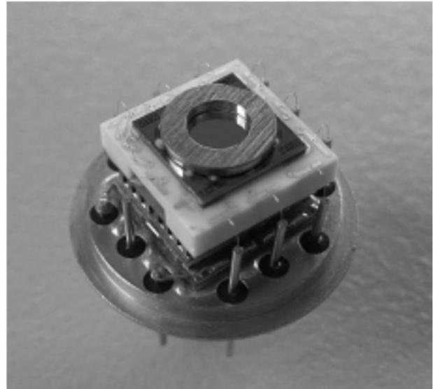
**Figure 1:** KETEK: x-ray detector
