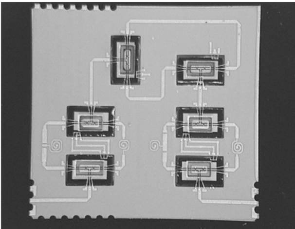
**Figure 12:** Thales: 3-bit phase shifters for phased array antenna
