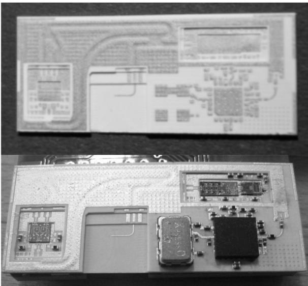
**Figure 22:** VIA/IMST: 77 GHz Radar Front end, Substrate and assembled package
