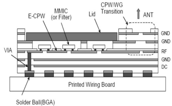
**Figure 9:** NEC: Schematic of the NEC 60 TR module
