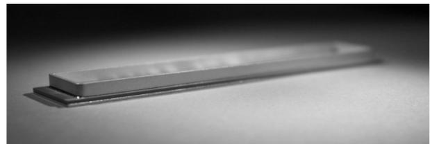
**Figure 14:** EADS: LTCC T/R Package
