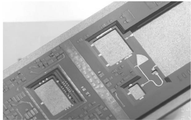
**Figure 13:** TNO: Design of a LTCC Transmit Receive Module
