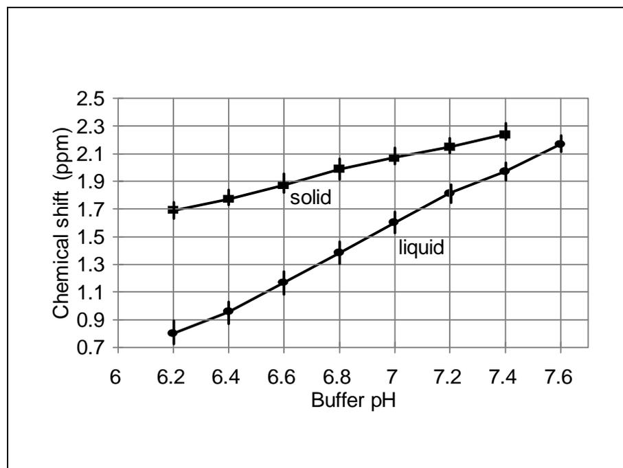
Figure 1: Chemical shift of ortho-phosphate peak recorded at  $-40\text{ }^{\circ}\text{C}$  with respect to different proton activities of buffers determined at  $22\text{ }^{\circ}\text{C}$ . Different shifts were recorded when the buffer containing phosphate was frozen, pulverised and than mixed with cold buffered methanol (■); or simply mixed with cold methanol to the final concentration of 60% v/v (●).
