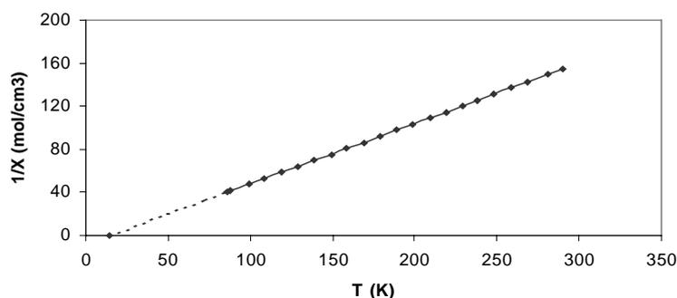
**Figure 2.** Magnetic susceptibility measurement of  $(\text{NH}_3\text{OH})_3\text{CrF}_6$ .
