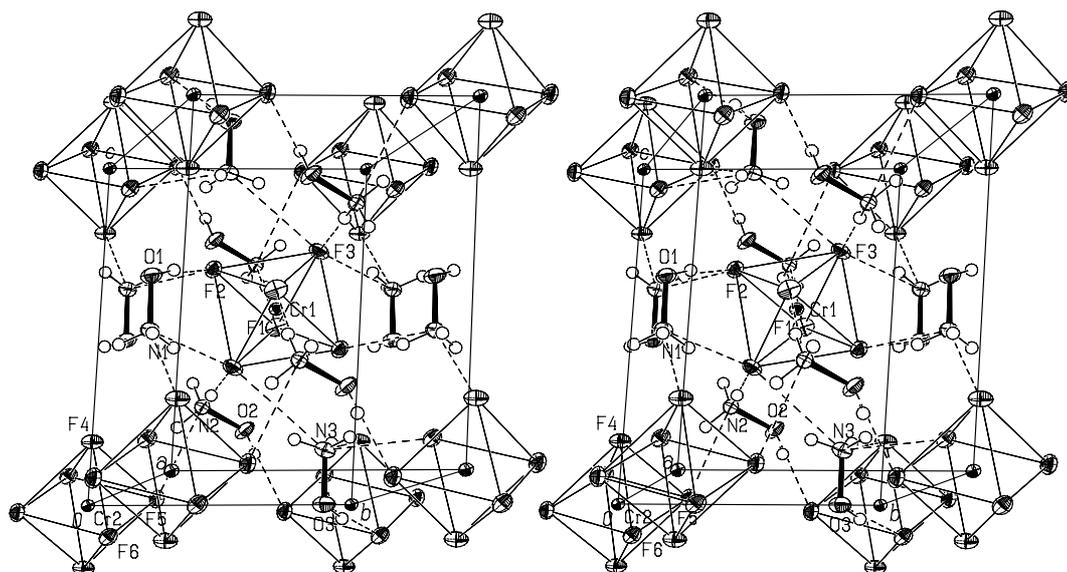
**Figure 3.** Stereoscopic picture of the  $(\text{NH}_3\text{OH})_3\text{CrF}_6$  unit cell.
