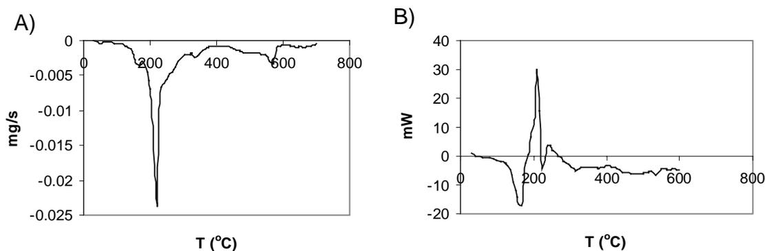
**Figure 1.** Thermal analysis of (NH<sub>3</sub>OH)<sub>3</sub>CrF<sub>6</sub>: A) DTG (Derivative Thermogravimetry), B) DSC (Differential Scanning Calorimetry).
