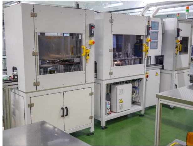
Fig. 2 Modular EoL quality inspection system
