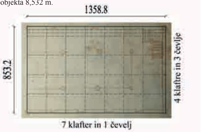
Slika 10: Izris tlorisnih mer v današnjem metričnem sistemu v primerjavi s takratnimi. Figure 8: Floor plan measurements in today's metrical system compared with the then measurements.
