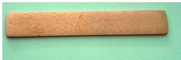
**Figure 3.** Pitting corrosion on a copper strip
