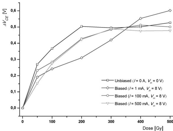
**Figure 2:** Change in the mean serial transistor's minimum dropout voltage in the voltage regulator L4940V5 under the influence of  $\gamma$ -radiation ( $V_{out} = 4.9\text{ V}$ ,  $I_{out} = 400\text{ mA}$ ).
