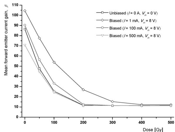
**Figure 3:** Change in the mean serial transistor's forward emitter current gain in the voltage regulator L4940V5 under the influence of  $\gamma$ -radiation ( $V_{out} = 4.9\text{ V}$ ,  $I_{out} = 400\text{ mA}$ ).
