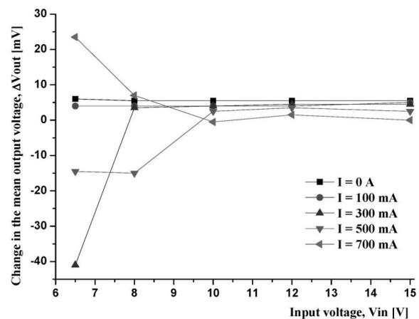
**Figure 8:** Relative line regulation characteristics of the unbiased voltage regulators L4940V5 after deposition of the total dose of  $\gamma$ -radiation of 300 Gy( $\text{SiO}_2$ ) (bias conditions:  $V_{in} = 0$  V,  $I = 0$  A).
