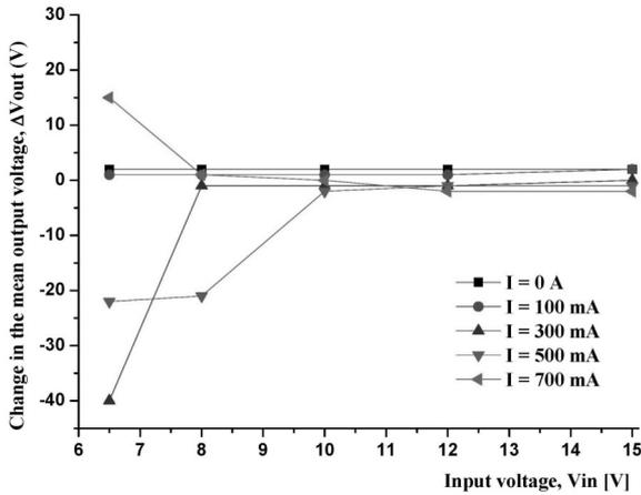
**Figure 9:** Relative line regulation characteristics of the biased voltage regulators L4940V5 after deposition of the total dose of  $\gamma$ -radiation of 300 Gy( $\text{SiO}_2$ ) (bias conditions:  $V_{in} = 7 \text{ V}$ ,  $I = 100 \text{ mA}$ ).
