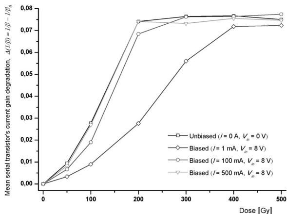
**Figure 4:** Change in the mean serial transistor’s current gain degradation in the voltage regulator L4940V5 under the influence of  $\gamma$ -radiation ( $V_{out} = 4.9\text{ V}$ ,  $I_{out} = 400\text{ mA}$ ).
