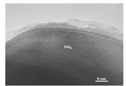
**FIGURE 3.** Transmission electron micrograph of an AlOOH-coated  $TiO_2$  NP (Courtesy of dr. G. Dražić).
