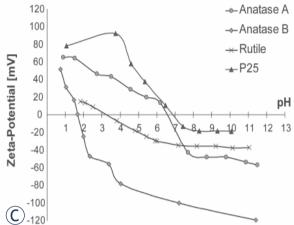
**FIGURE 1.** Field emission electron micrographs of different  $TiO_2$  powders: A) Anatase A (Sigma 637254), B) Anatase B (Sigma T8141); C) Zeta-potential of these two powders, Rutile (Sigma 637262) and P25 (Degussa).
